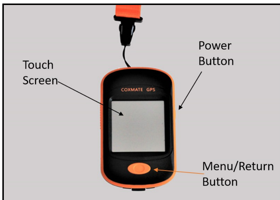
1. Button configuration with full touch screen
